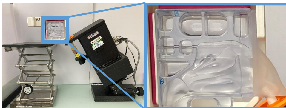
Figure 1: Deposition testing bench and nasal cast
