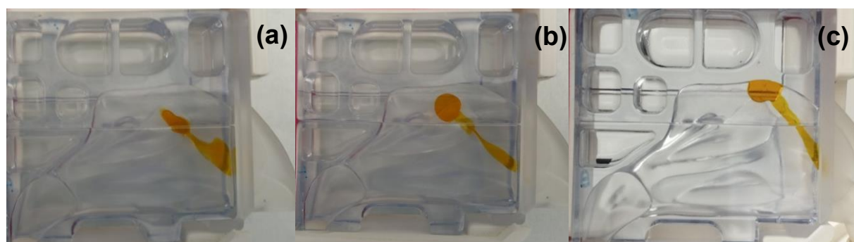
Figure 4: Illustration of the discrepancies between repetitions – Boundary effect of the nasal cast parting line. (a) and (b): two repetition of the same border case, 47 and 83% respectively. (c):deposition pattern with optimal orientation, 90% in olfactory area
