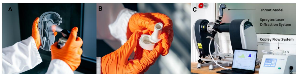
Figure 1 – (A) Two-piece 3D printed anatomical throats with sagittal dissection, sealing cord and interfaces for Malvern Spraytec and RS01 DPI. Coating of internal surfaces with silicone oil to reduce re-entrainment of particles on wall impaction. (B) RS01 DPI device with Size 3 HPMC capsule inserted. (C) Test setup with 3D printed anatomical throat, Malvern Spraytec with Inhalation Cell, Copley TPK 2000-R Critical Flow Controller, Copley HCP5 Vacuum Pump and in-line TSI-4043 mass flow meter
