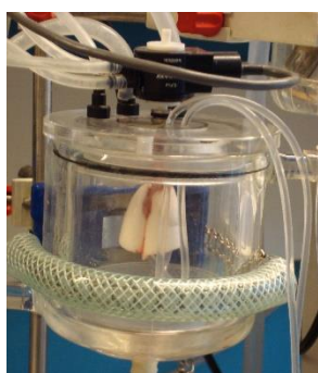
Figure 2- A prepared isolated, perfused and ventilated rat lung (IPL); Before aerosol exposures, the Hans Rudolph pneumotachograph was removed and the tracheal catheter of the IPL was connected to the PreciseInhale at the exposure block (Figure 1, EB).
