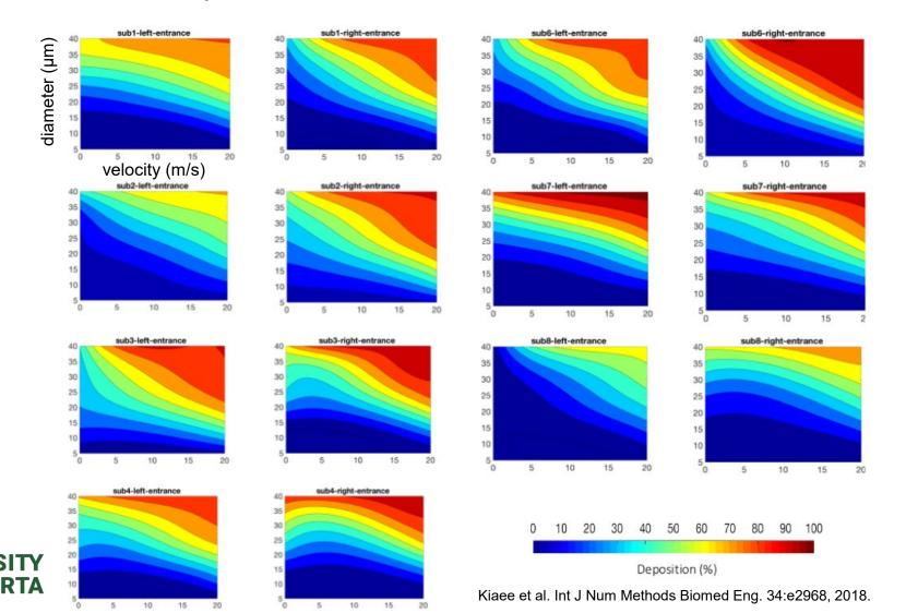
• <u>Turbinates Deposition</u> (avg. over cone angle, spray direction, injection location):
