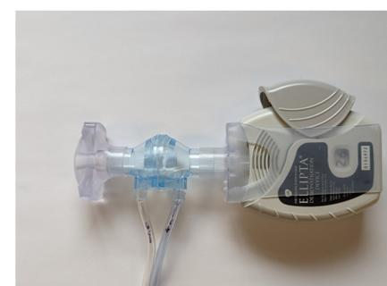
**Figure 3: Ellipta\* DPI with flow sensor/adaptor**
