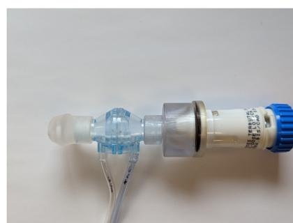
**Figure 3: Turbuhaler\* DPI with flow sensor/adaptor**
