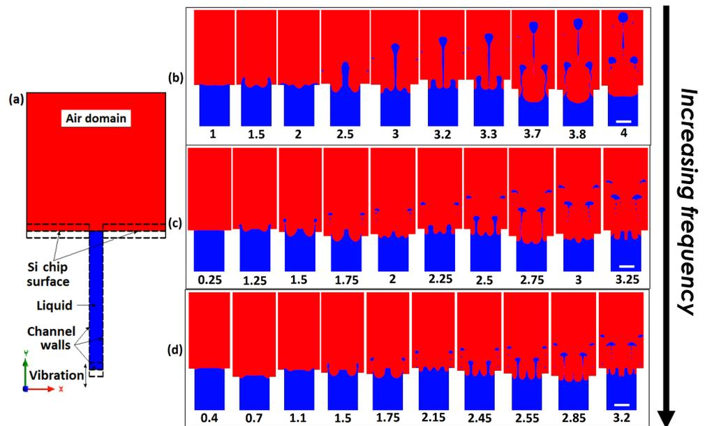
Figure 2: (a) CFD 2D model of the PALM and the dashed lines vibrate vertically. 2D CFD snapshots for ligament formation and their breakup into droplets being ejected from a microchannel filled with water vibrated at different forcing frequencies and amplitudes. At (b) 1 MHz & 3.25 μm, (c) 2.5 MHz & 2.5 μm, and (d) 4 MHz & 2 μm. The values beneath every simulation represent the number of cycles of vibrations. All white bars are 10 μm.
