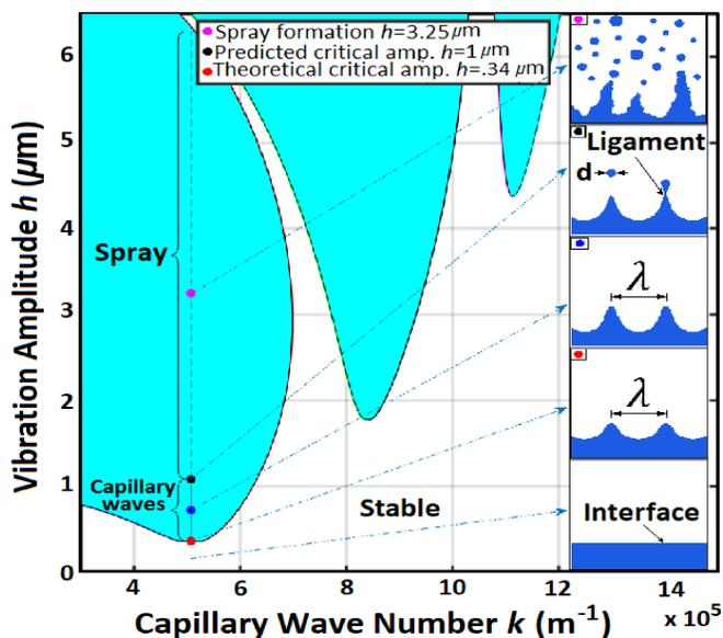
Figure 1: The damped Mathieu stability chart for liquid water actuated at 1 MHz. Cyan (unstable), white (stable), and the minimum (red) point indicates the theoretical critical threshold (0.34 μm) for droplet ejection. Insets are schematic representations of the spray formation stages starting from a flat interface followed by generation of capillary waves.
