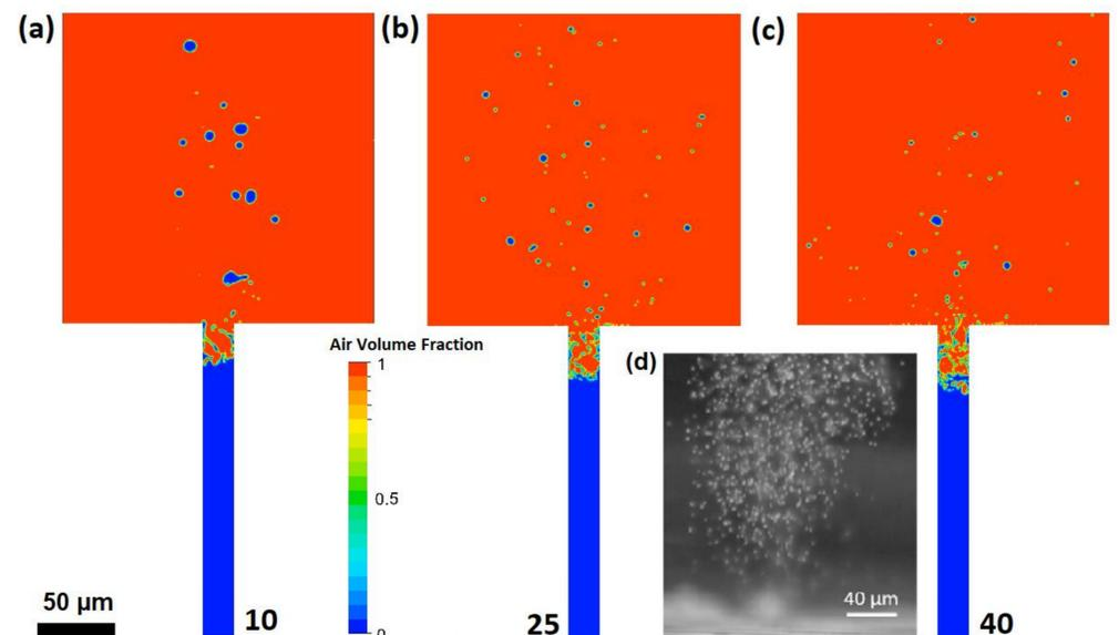
Figure 3: 2D CFD snapshots for spray formation at (a) 1 MHz & 3.25 μm, (b) 2.5 MHz & 2.5 μm, and (c) 4 MHz & 2 μm. (d) Snapshot of droplets as they leave the microfluidic chip. Recorded at 30,000 fps.
