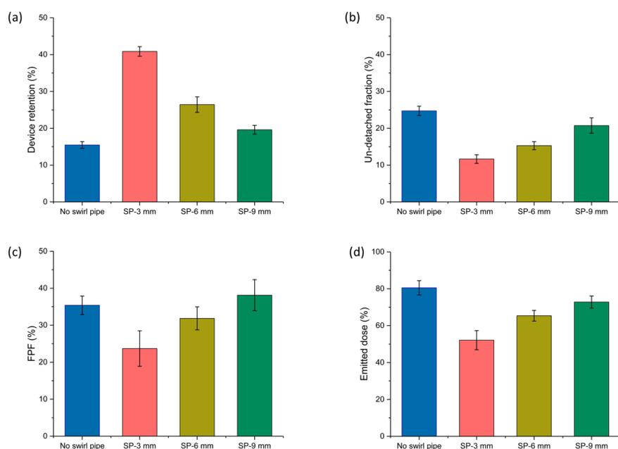
Figure 2 The aerosolization performance including (a) drug retention in the device, (b) un-detached drug fraction in pre-separator, (c) fine particle fraction, and (d) emitted dose
