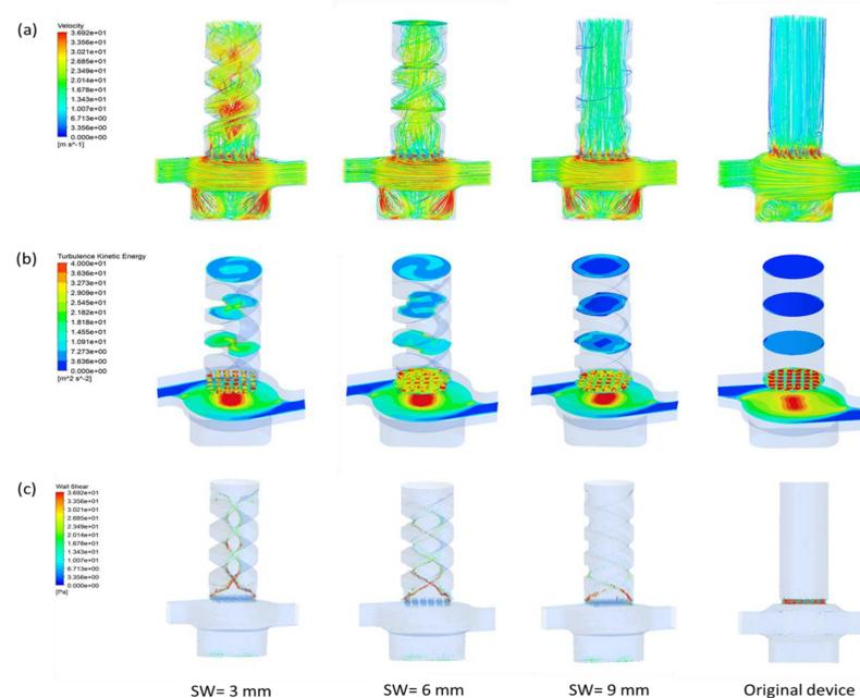
Figure 3 Contour maps of (a) airflow trajectories, (b) turbulent kinetic energy, and (c) wall shear in the inhalers with different swirl pipe designs
