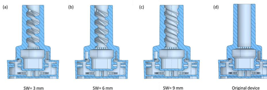
Figure 1 Illustration of 3D models of the inhalers with different swirl pipe designs
