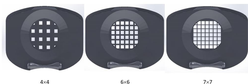
Figure 1 Front view of grid mesh of modified 3D inhalers
