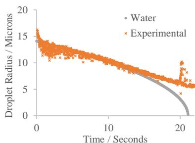
**Figure 4.** Size of a droplet originally made of Formoterol Fumarate Dihydrate dissolved in ethanol (orange Xs) injected into an airflow with a relative humidity of 81%. The grey line is a model of the size change of a water droplet injected into an airflow with a relative humidity of 81%.
