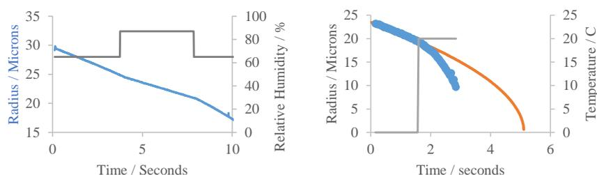
**Figure 2.** The rapid change of relative humidity (left) and temperature (right) that a single levitated water droplet in a CK-EDB experiences. The orange line on the right indicates a model prediction for an evaporating water droplet into air set at a temperature of 0°C and a relative humidity of 0%.
