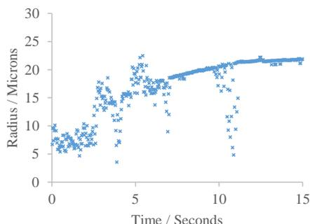
**Figure 3.** The dissolution of a sodium chloride particle. The relative humidity is increased from dry to >80% at 0 seconds (<0.1 seconds for the RH change to occur). When the particle is non-spherical, it is not accurately sized. It takes 7 seconds for the dry sodium chloride particle to completely dissolve into a spherical droplet.
