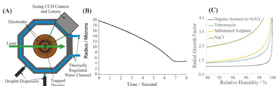
**Figure 1. (A) Key components of the CK-EDB. (B) The measured radius of the droplet as a function of time. This data is then used to calculate (C), the hygroscopic properties.**
