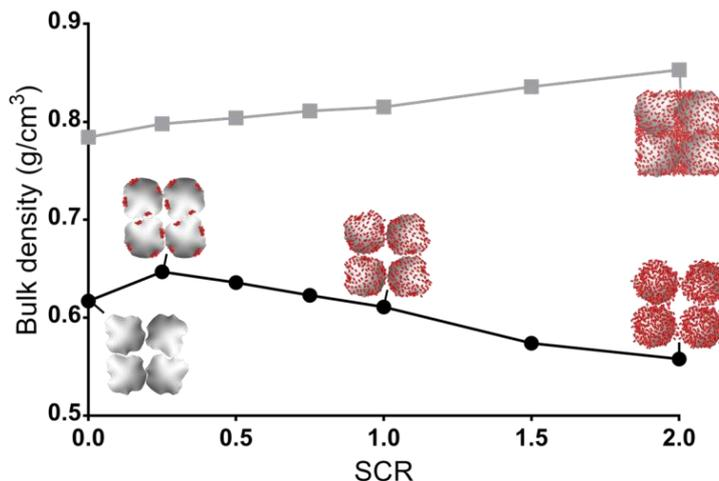
Figure 3 – Bulk density used as a parameter to explain the mixture structure for un-consolidated mixtures (black line) and after consolidation (30 kPa, greyed line)
