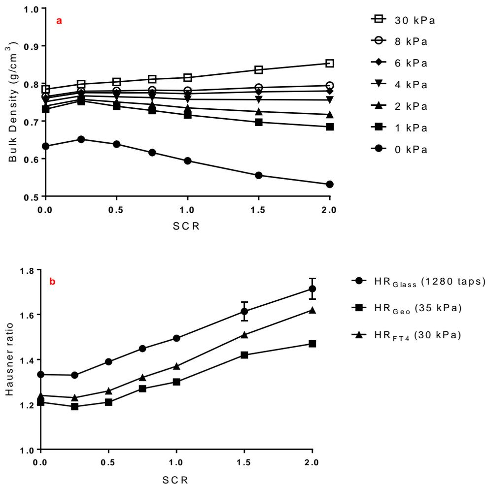
**Figure 2 – a) Mixtures exposed to different levels of compression (using FT4 Powder rheometer) and - b) Hausner ratios (obtained from three different tests), plotted versus Surface coverage ratio (SCR). Average values (n=3) with standard deviation, some too low to be visible.**
