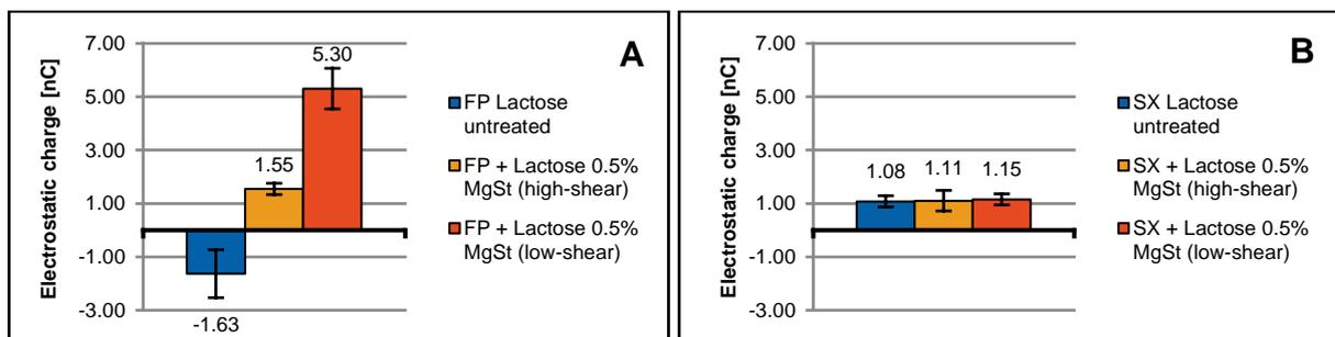
**Figure 3** Dynamic charge measurement with Breezhaler® device for FP (A) and SX (B) blends (n=5 capsules).
