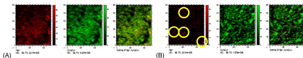
**Figure 1** ToF-SIMS micrographs at scanning area of 500µm×500µm for (A) Lactose 0.5% MgSt (high-shear) and (B) Lactose 0.5% MgSt (low-shear). Red = Signal for MgSt (Mg<sup>+</sup>). Green = Signal for Lactose (C<sub>3</sub>H<sub>5</sub>O<sub>2</sub><sup>+</sup>). Orange = Overlay.
