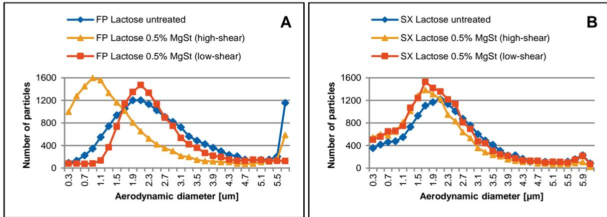
**Figure 2** SPAMS Aerodynamic particle size distribution histogram of FP (A) and SX (B) blends with lactose untreated, 0.5% MgSt (high- and low-shear), respectively. The plot shows the total number of particles measured (APIs and excipients).
