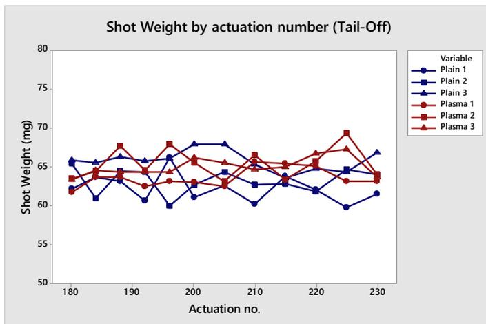
Figure 3 – Shot weights for tail-off testing
