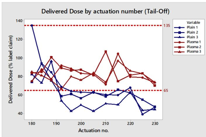
Figure 2 – Tail-off characteristics for Plasma-treated and Plain canisters, using Delivered Dose
