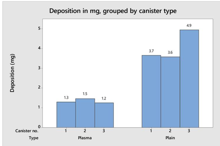
**Figure 4 – Drug deposition on canister walls**
