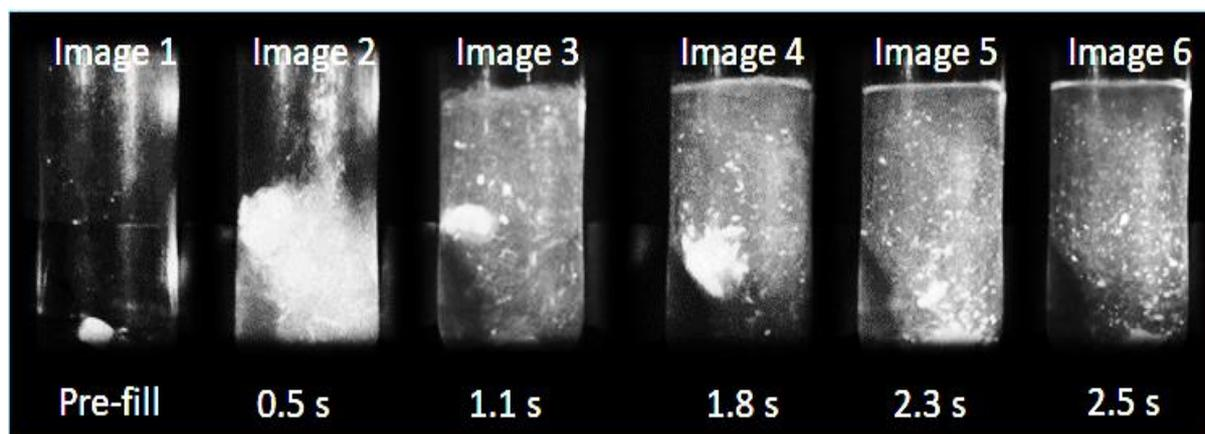
**Figure 1. Images Taken During Propellant HFA 134a Filling of a PET Vial Containing an SS Opt2Fill Tablet.**
