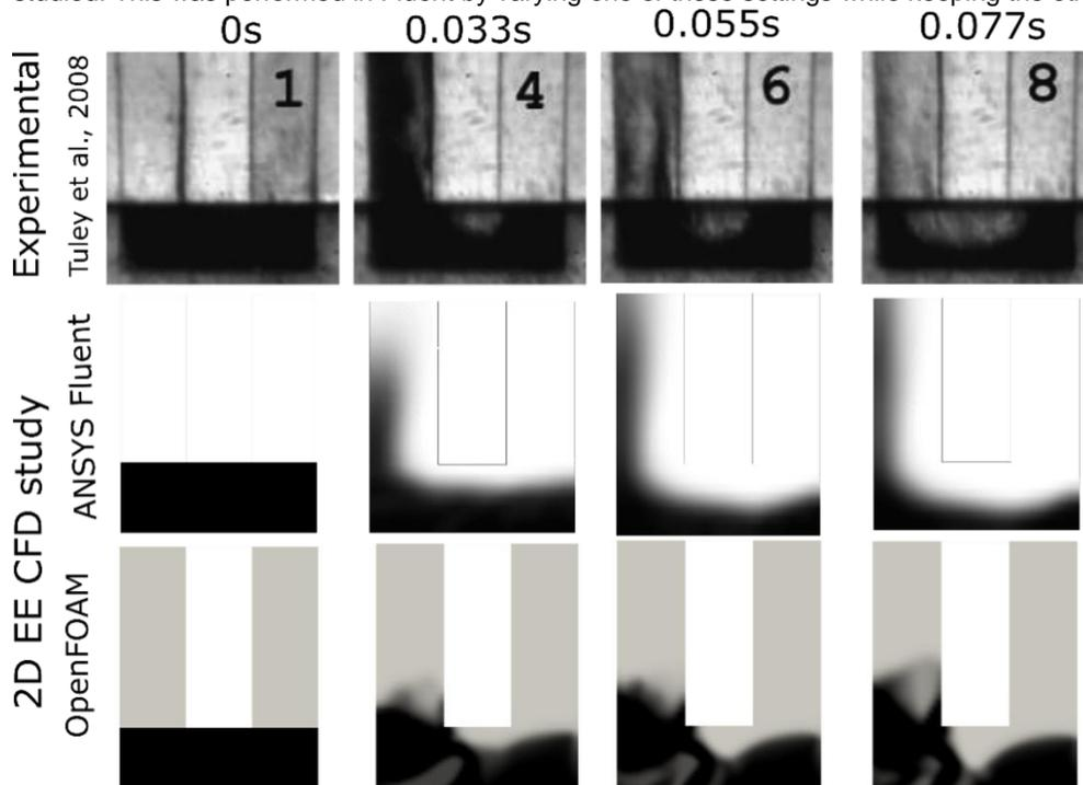
Figure 1 - Comparison of experimental results from Tuley *et al.* [7] with CFD simulation results from ANSYS Fluent [6] and OpenFOAM [8]. This comparison is for glass powder (mean particle  $d = 45 \mu\text{m}$ ). Time before the beginning of emptying excluded.
