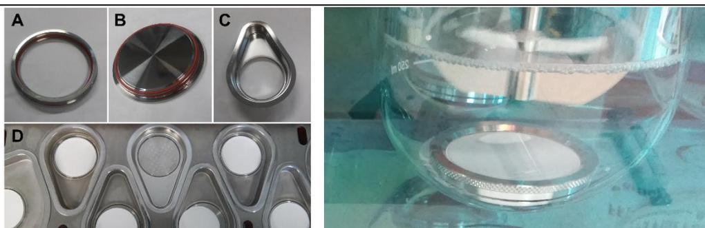
Figure 1 – Left: Modified NGI. A – Securing ring of the membrane holder; B – stainless steel collector and membrane holder; C – Dissolution cup; D – NGI with dissolution cup after actuation. Right: Dissolution vessel with membrane holder.
