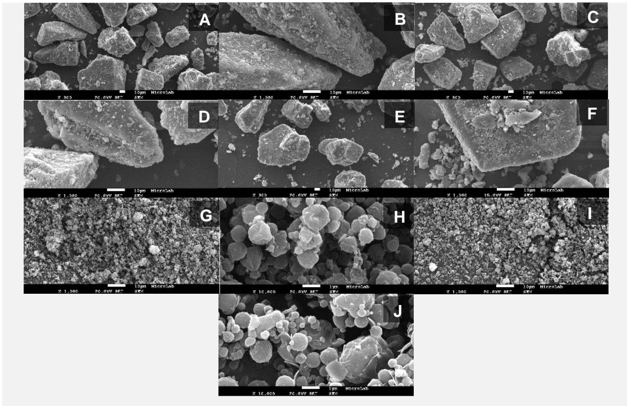
Figure 2 – SEM micrographs for blends with 5, 10 and 15% fines, B<sub>1</sub> (A and B), B<sub>2</sub> (C and D) and B<sub>3</sub> (E and F), x300 and x1000 respectively; and for composites containing trehalose and raffinose, C<sub>1</sub> (G and H) and C<sub>2</sub> (I and J), x1000 and x 10 000 respectively; at 20 kV.
