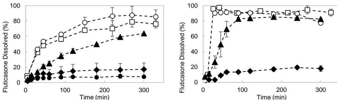
Figure 4 – Left: Dissolution profile in the paddle over disk apparatus of composites C<sub>1</sub> (○) and C<sub>2</sub> (□), and of blends B<sub>1</sub> (▲), B<sub>2</sub> (◆) and B<sub>3</sub> (●); right: dissolution profile in the paddle apparatus of hand filled capsules filled with of composites C<sub>1</sub> (○) and C<sub>2</sub> (□), and of blends B<sub>1</sub> (▲) and B<sub>2</sub> (◆). Each profile is given by two replicates.
