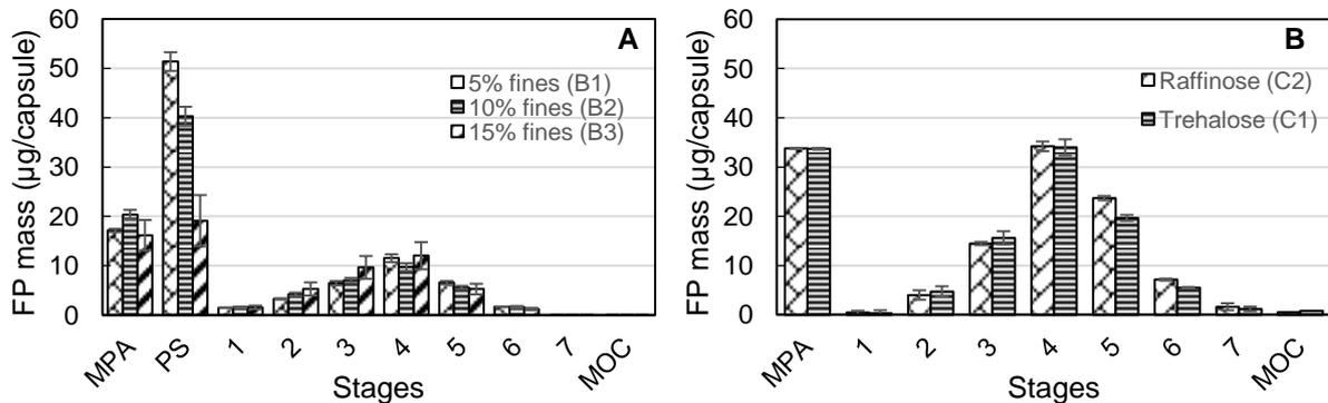
Figure 3 – API deposition at dose plate for blends B<sub>1</sub>, B<sub>2</sub> and B<sub>3</sub> (A) after 3 repetitions of 10 actuations at 40 L/min using PowdAir inhaler; for composites C<sub>1</sub> and C<sub>2</sub> (B) after 3 repetitions of one actuation at 40 L/min using Plastiapi Monodose inhaler. MPA is mouth piece adapter and induction port; PS is pre-separator and MOC is micro-orifice collector.
