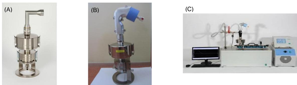
Figure 1 – Set up equipment used during the course of this work: (A) – IP + FSI (image from Copley Scientific website), (B) AIT + FSI, (C) – BRS + AIT + FSI (image from Copley Scientific website)
