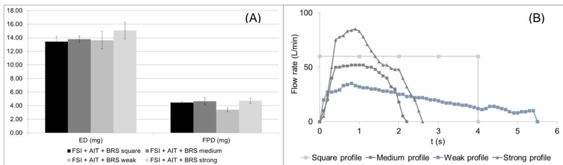
Figure 3 – (A) ED and FPD results obtained by gravimetric FSI with the Plastiapae device, where the error bars correspond to one standard deviation; (B) Different inhalation profiles: square, medium, weak and strong.
