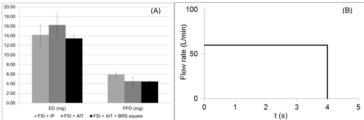
Figure 2 - (A) ED and FPD results obtained by gravimetric FSI with the Plastiapae device, where the error bars correspond to one standard deviation; (B) Square wave profile (representative of a vacuum profile).
