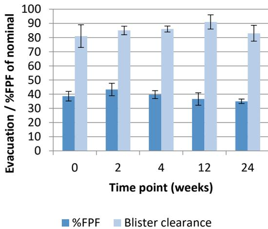
**Figure 3:** Gravimetric FSI stability results- evacuation and percentage fine particle fraction (%FPF)
