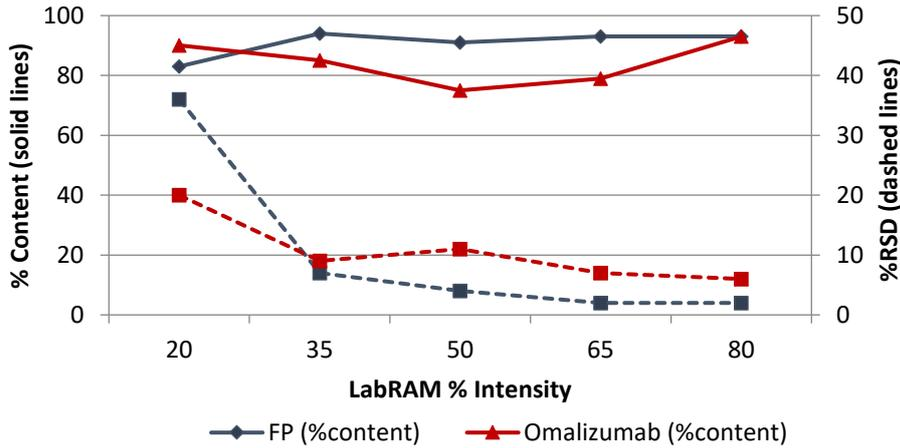
**Figure 1:** Process optimisation – content homogeneity assessment at a range of LabRAM blending intensities (mean of 5 content uniformity replicates)
