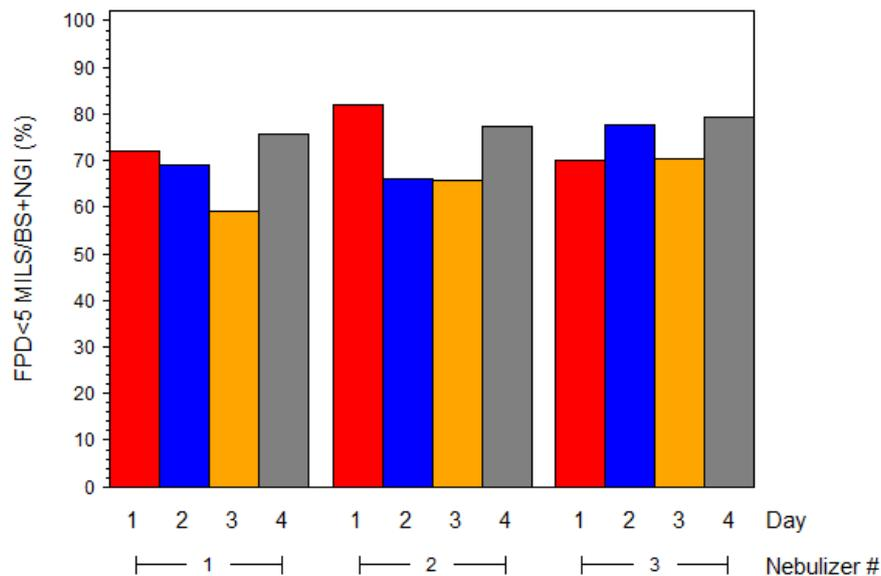
**Figure 2 Values of FPD<sub><5µm</sub> by MILS Procedure Expressed as a Percentage of FPD<sub><5µm</sub> by BS + NGI Compendial Procedures for Each Nebuliser Tested on Each Day of the Investigation**
