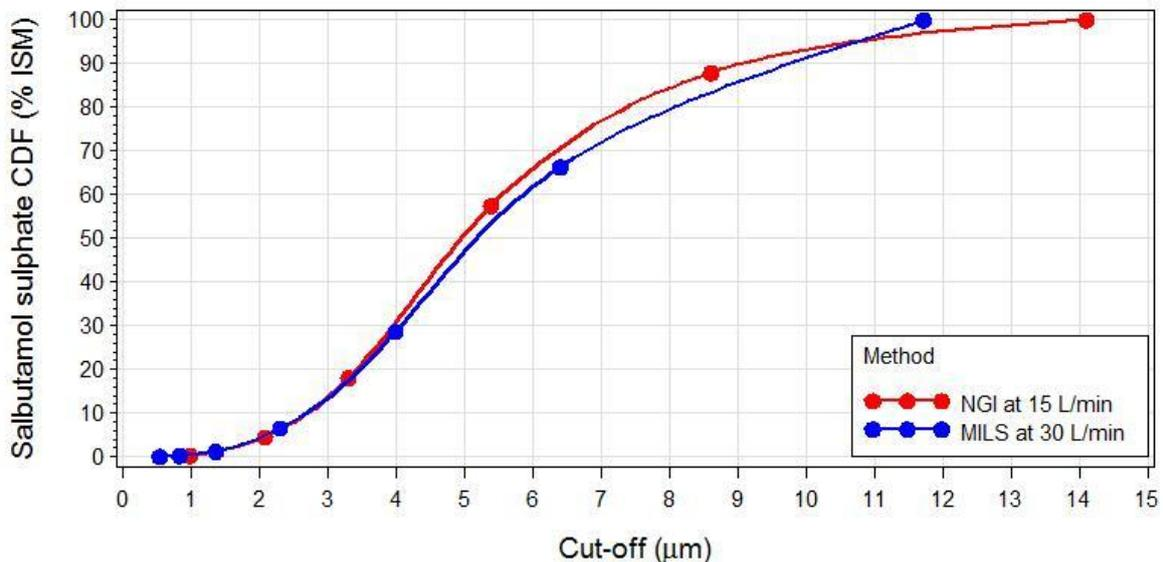
**Figure 3 Cumulative Size Distributions for Salbutamol Sulphate as Percentage of Impactor Sized Mass (ISM = Sum of Drug Depositions on S2 to the MOC) by Compendial (NGI) and MILS Configurations for the eFlow® Rapid Vibrating Membrane Nebuliser**
