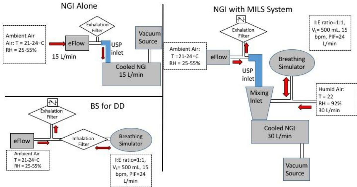
**Figure 1 Configurations for the Compendial Procedures (BS for DD and NGI Alone) and for the NGI with MILS Methodology**
