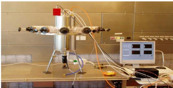
Figure 5 - A first novel functional fully equipped nose-only aerosol exposure system for in-vivo use
