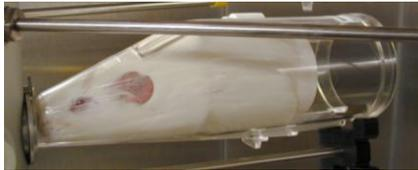
Figure 2 - A rat in a commercially available restraining tube for nose-only inhalation exposure.
