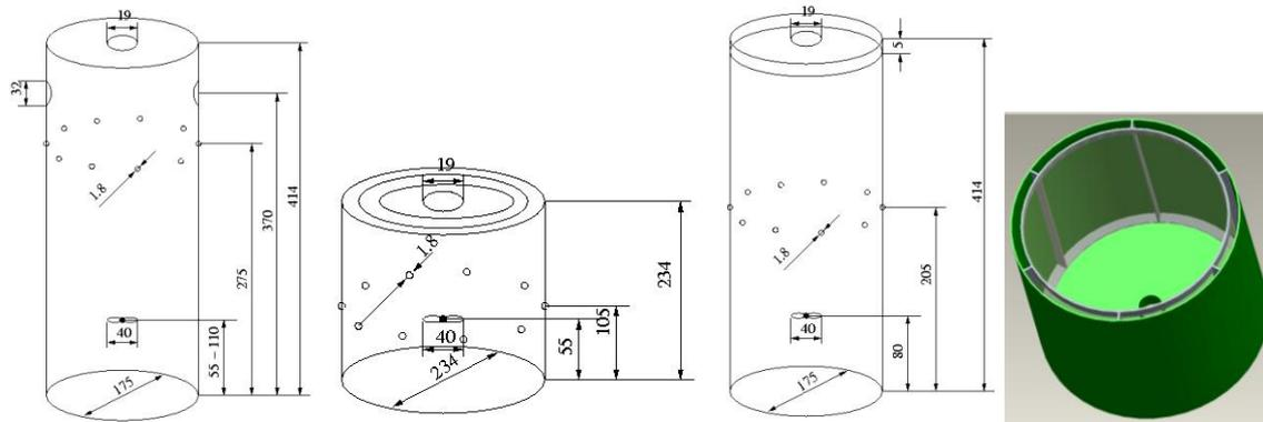
Figure 3 - Three different theoretical models and a plot of the hollow walls of the closed exposure chamber that were evaluated using computational fluid dynamic simulations.
