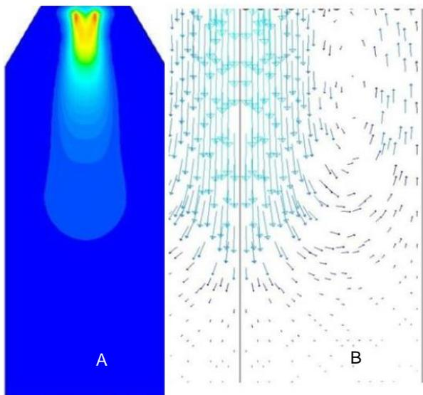
Figure 4 - A. Contour plot of the turbulent kinetic energy in the holding chamber. B. Illustration of swirls in the air velocity vectors
