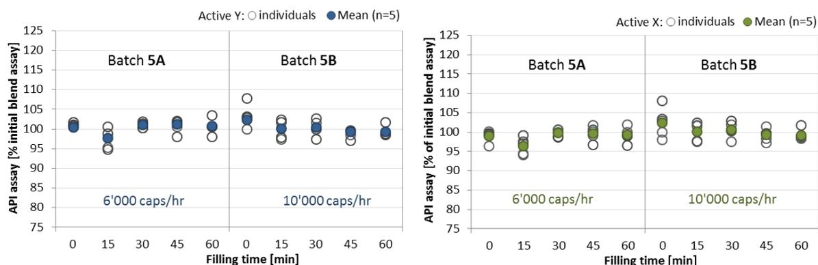
Figure 5 – Capsule content results of the combination batch filled with the 2.8mm Ø dosators at different speeds
