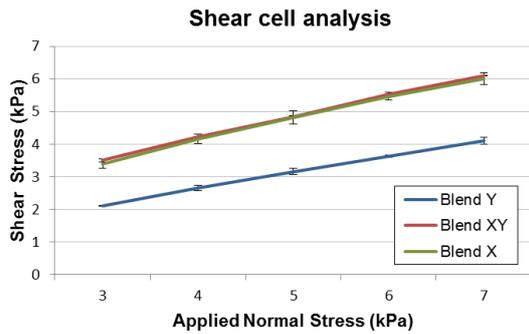
Figure 3 – Shear cell analysis of the DPI blends
