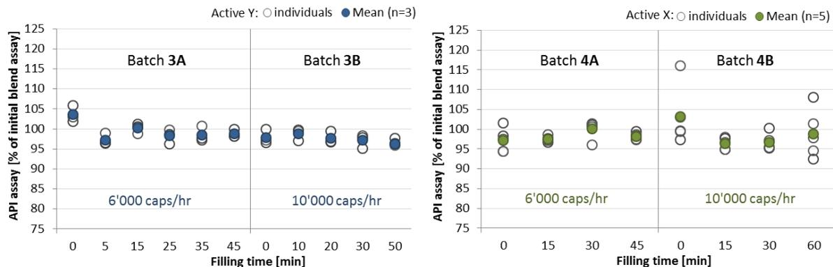
Figure 4 – Capsule content results of the single API batches filled with the 2.8mm Ø dosators at different speeds
