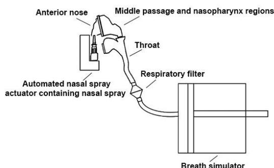
Figure 1. Schematic diagram of experimental setup for the realistic *in vitro* nasal deposition studies
