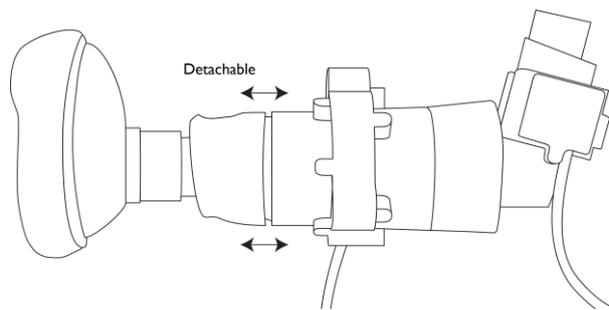
**Figure 2: Facemask Datalogger assembly**
