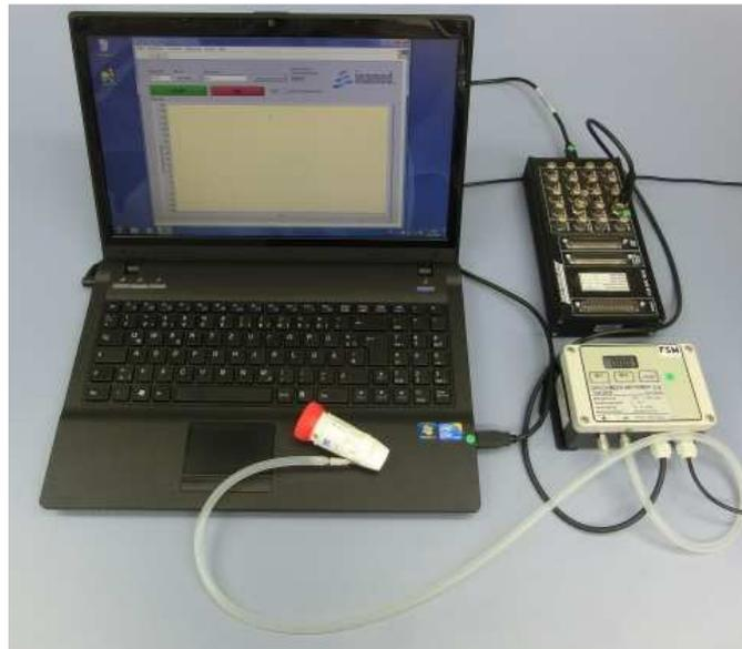
Figure 1: Assembled measurement kit with Turbohaler
