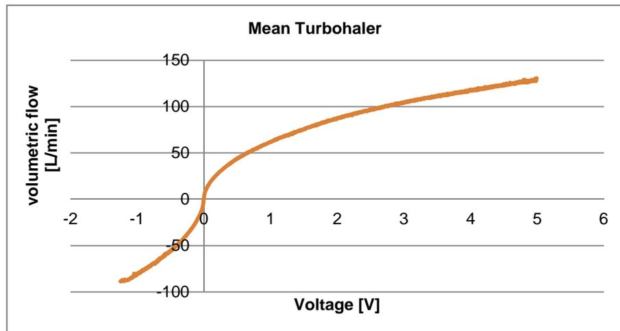
Figure 3: Example calibration curve of the Turbohaler
