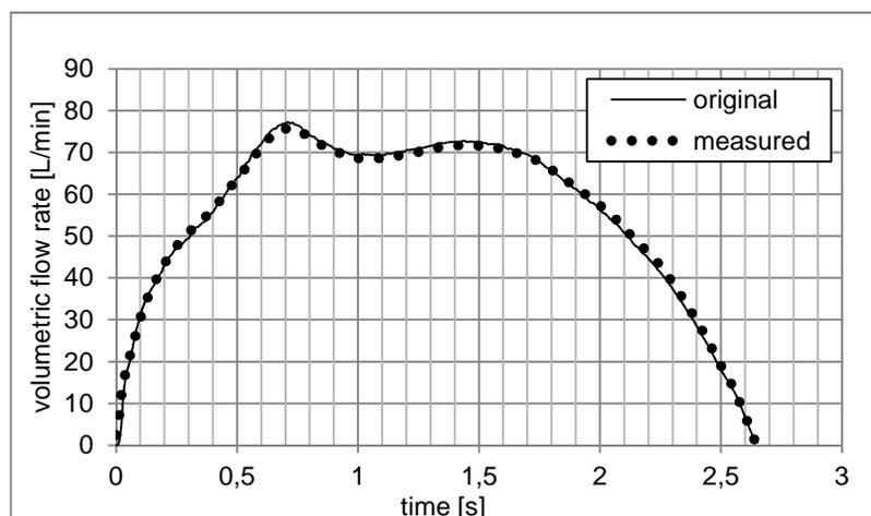
Figure 4: Comparison of measured values by the software to original values
