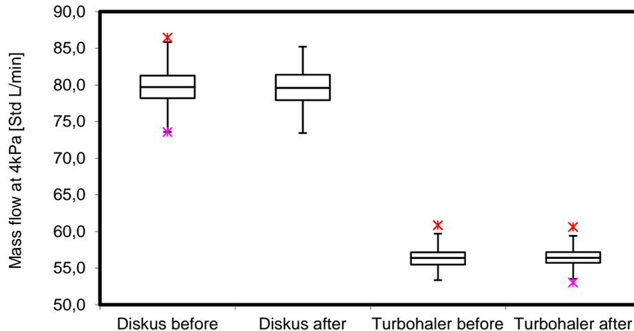
Figure 3: The flow rate at 4 kPa, before and after the modification of the device was Diskus before 79.8 L/min  $\pm$  2.6 L/min and after 79.6 L/min  $\pm$  2.5 L/min and Turbohaler before 56.3 L/min  $\pm$  1.2 L/min and after 56.4 L/min  $\pm$  1.2 L/min (mean and SD of 150 devices each).
