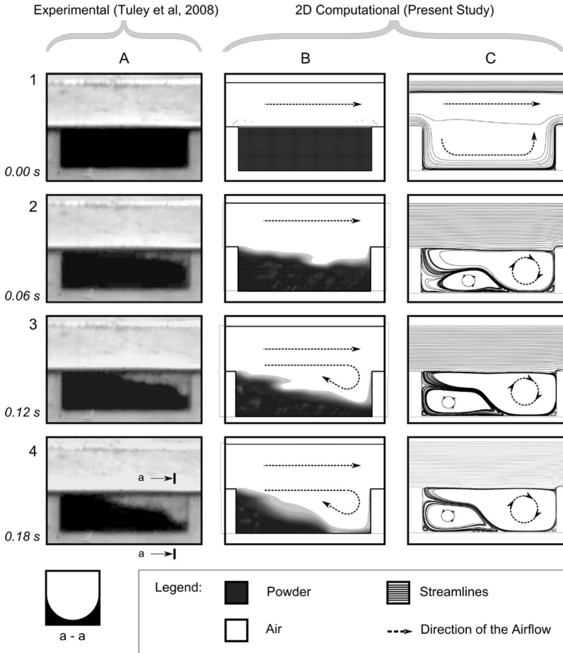
Figure 2 Comparison between experimental [3] and computational results for geometry *A*. Columns show different types of studies: *A* – experimental, *B* – computational multiphase (air and powder) and *C* – computational single-phase (air only). Rows correspond to different moments in time; experimental time before the start of evacuation was excluded.
