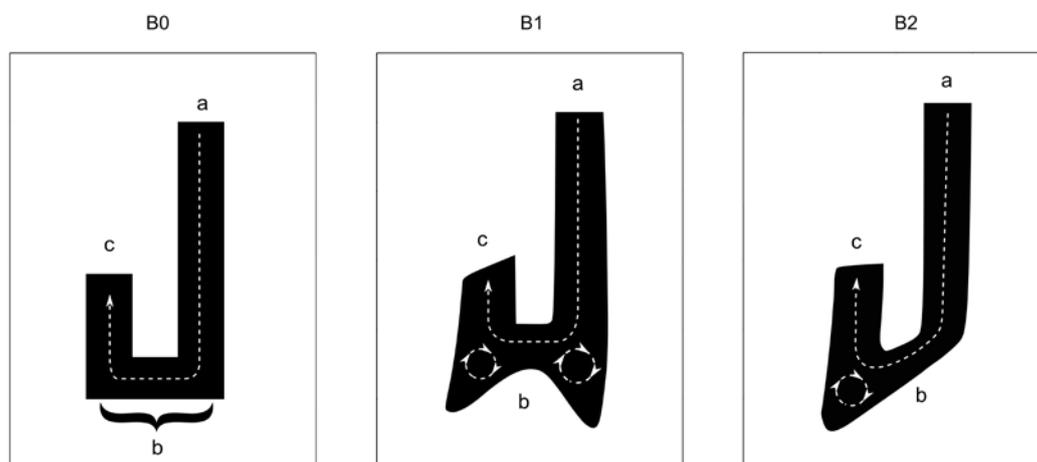
Figure 3 Standard (B0) and optimised for flow rate independence (B1 and B2) geometries. Detail *a* – air inlet, *b* – powder bed and *c* – outlet. Arrows indicate the direction of the airflow and recirculations.
