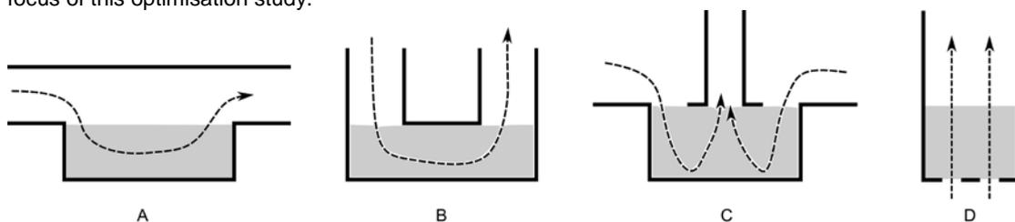
Figure 1 Simplified entrainment geometries encountered in industry and academic research: A – shear force entrainment [1]; B, C and D – gas-assisted entrainment [2, 3, 4, 5]. Gray areas indicate the powder, arrows – direction of the flow.
