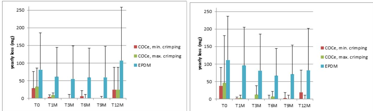
Figure 1 - Leak rate testing of various configurations of MDIs (n=25) with different sealing gaskets containing HFA with 15% w/w (left) and without (right) ethanol at 20°C crimped at different parameters. Bars represent max & min values observed.
