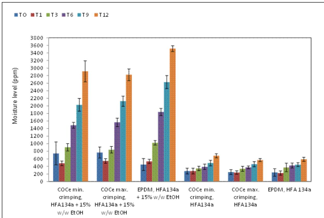
Figure 2 - Moisture level results of various configurations of MDIs (n=15) with different sealing gaskets containing HFA with & without ethanol and crimped at different parameters, tested using Karl Fisher. Error bars represent +/- one standard deviation.
