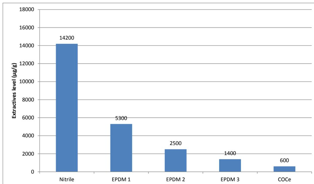
**Figure 3** - Extractable levels measured in various gasket sealing materials assessed by HPLC and GCFID
