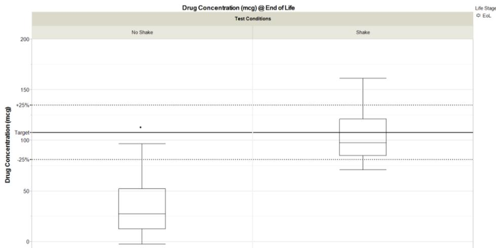
**Figure 3. Detailed view of end of life DCU performance for Product A (no excipients) with and without shaking.**
