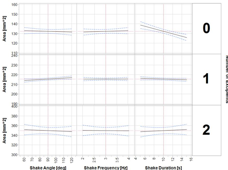
**Figure 1: Consolidated optical spray pattern sensitivity profiles for the three (3) tested pMDI products (identified by the number of excipients) as a function of shaking. Auto-scaled y-axes were used to accommodate the different spray pattern area ranges for the products.**
