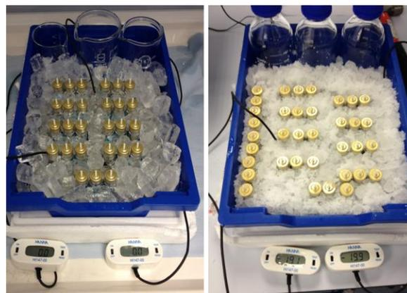
Figure 2. Cooling baths used for low temperature measurement
