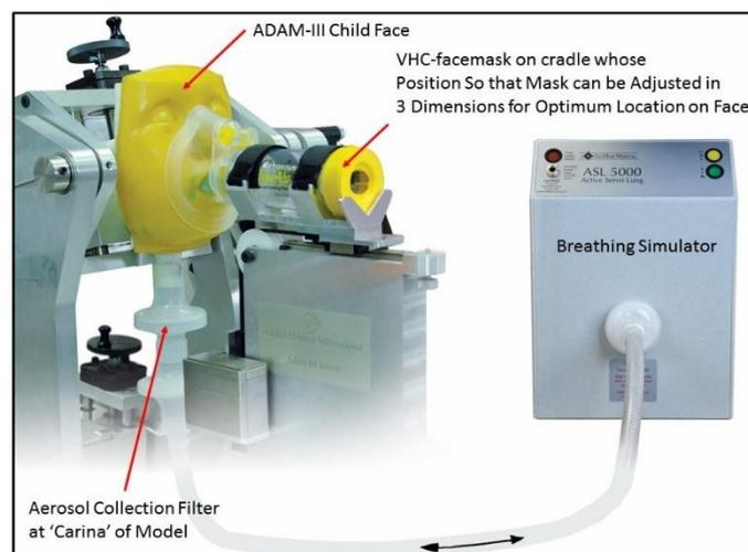
Figure 2: ADAM-III Small Child Face/Oropharynx Model with Breathing Simulator, Showing Position of Filter at Distal End of Oropharynx Mimicking Delivery of Medication at the Carina
