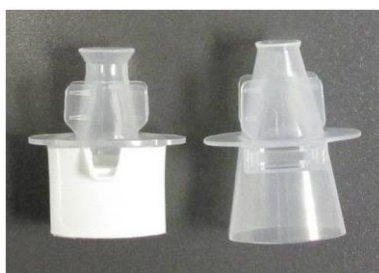
Figure 2 – Moulded adaptor plus short Flo-Tone without reed (left), and Flo-ToneCR prototype with rotated reed and flared mouthpiece (right).
