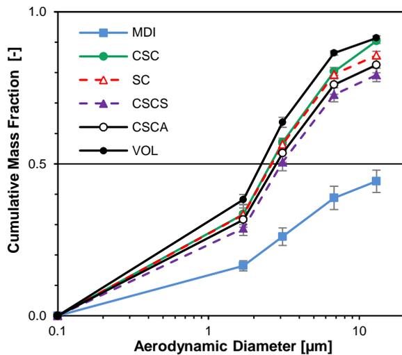
**Figure 1 - Cumulative mass fraction from the TEM of each device tested.**
