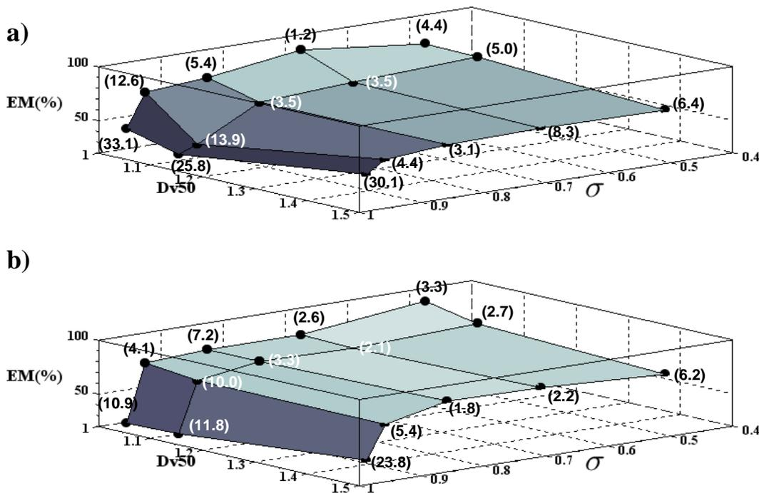
**Figure 1. Impact of changes on i) device blockage and ii) size of composite particles in the EM attribute: a) Fill weight of 20 mg/cavity; b) Fill weight of 40 mg/cavity. Data points represented are the mean value of N=3 replicates and values in brackets denote one standard deviation.**
