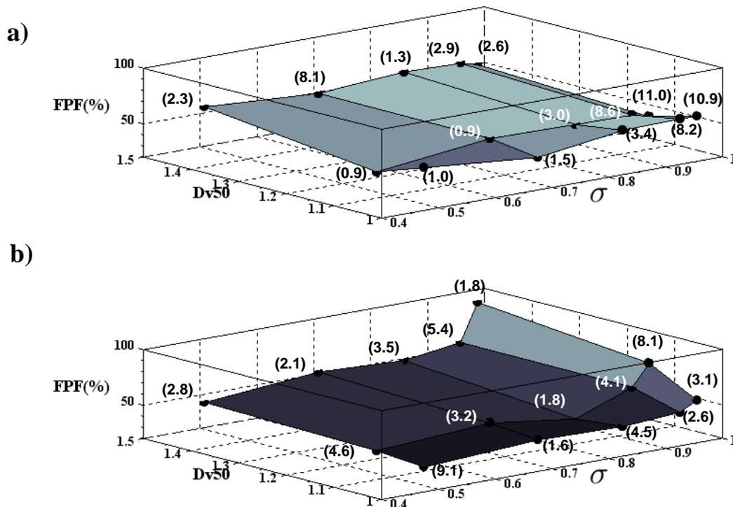
Figure 2. Impact of i) device blockage and ii) size of composite particles in the FPF attribute: a) Fill weight of 20 mg/cavity; b) Fill weight of 40 mg/cavity. Data points represented are the mean value of N=3 replicates and values in brackets denote one standard deviation.
