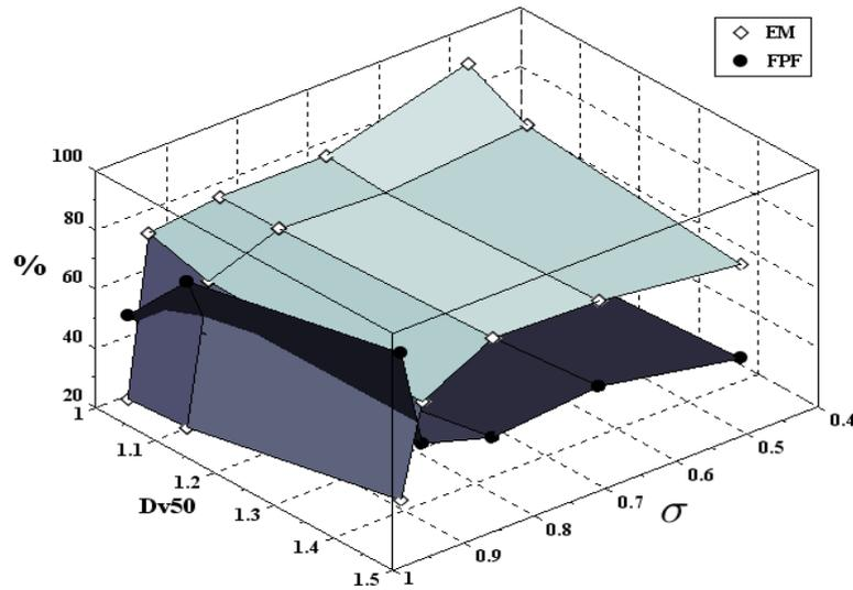
Figure 3. Exploration of the trade-off space between EM and FPF as a function of i) device blockage and ii) size of composite particles at the fill weight of 40 mg/cavity. Data points represented are the mean value of N=3 replicates. Standard deviation values corresponding to each EM and FPF data point are respectively presented in Figures 1b and 2b.
