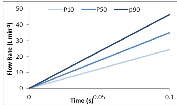
Figure 4 - Increase in flow rate between 0 and 0.1 secs for the P10, P50 and P90 inhalation profiles
