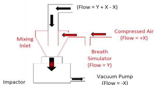
Figure 2- Schematic of impactor and breathing simulator set-up
