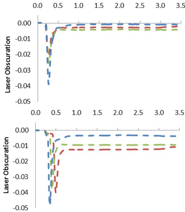
**Figure 5** - LiveShot evacuation profiles (pressure and laser obscuration) of (A) The NEXThaler device No-BAM variant and (B) The Control NEXThaler device, using the P10, P50 and P90 inhalation profiles (n=3)
