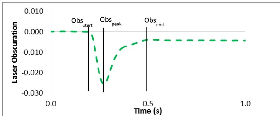
**Figure 6** - Dose Evacuation Profile using the No-Bam NEXThaler device with the P50 inhalation profile demonstrating the start ( $Obs_{start}$ ), peak ( $Obs_{peak}$ ) and end ( $Obs_{end}$ ) of the Laser Obscuration
