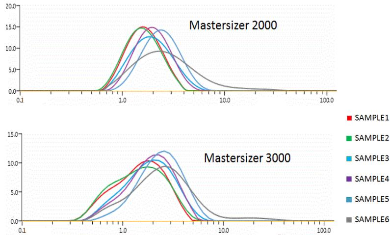
Figure 1 - PSD of Active A Samples 1 to 6 measured on the Mastersizer2000 and Mastersizer3000 instruments.
