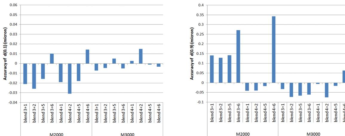
**Figure 5a and 5b - Accuracy of d(0.1) and d(0.9) for a range of blends of Active A on both instruments**
