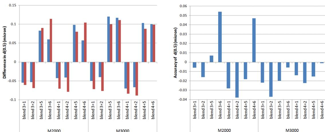
**Figure 4a - Theoretical  $d(0.5)$  shift (red bars) and the measured  $d(0.5)$  shift (blue bars) for a range of blends of Active A on both instruments**
