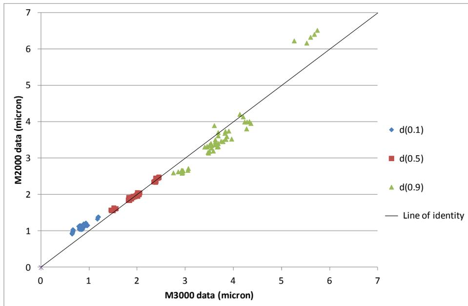
Figure 2 - Comparison of PSD data for Active A measured on the Mastersizer2000 and Mastersizer3000 instruments.
