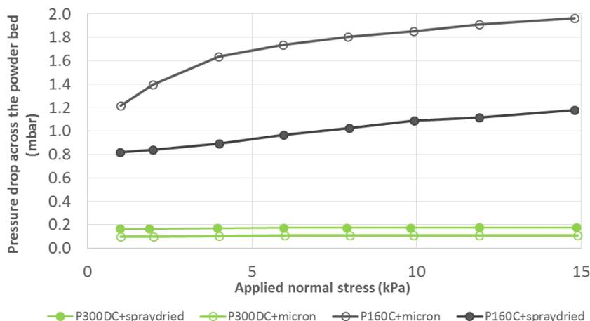
Figure 4: Air permeability of the adhesive mixtures
