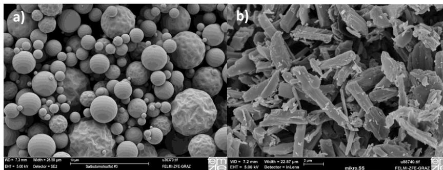
Figure 1 SEM images of micronized and spray dried salbutamol sulphate particles.
