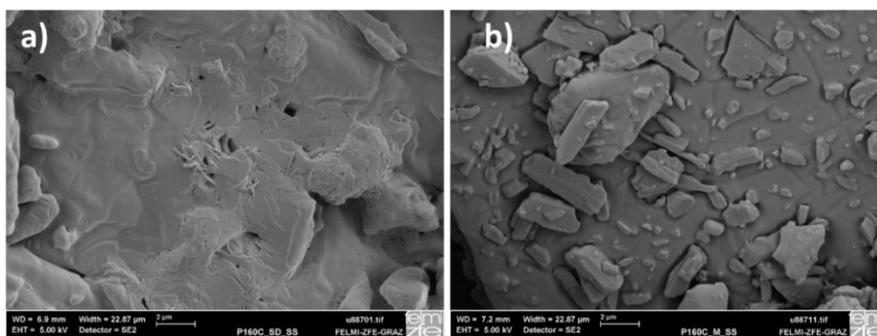
Figure 3: SEM images of adhesive mixtures containing P160C and a) spray dried and b) micronized salbutamol sulphate particles.
