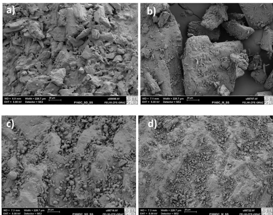
Fig. 2 SEM images of adhesive mixtures containing P160C with a) spray dried and b) micronized salbutamol sulphate particles and containing P300DC with c) spray dried and d) micronized salbutamol sulphate particles.
