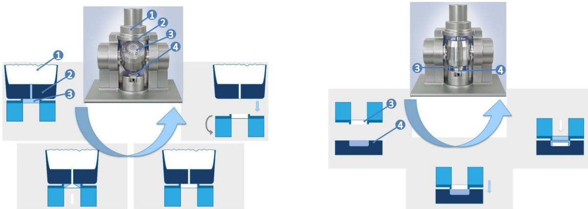
**Figure 2: Filling process; Left: filling of dosing chamber;**
