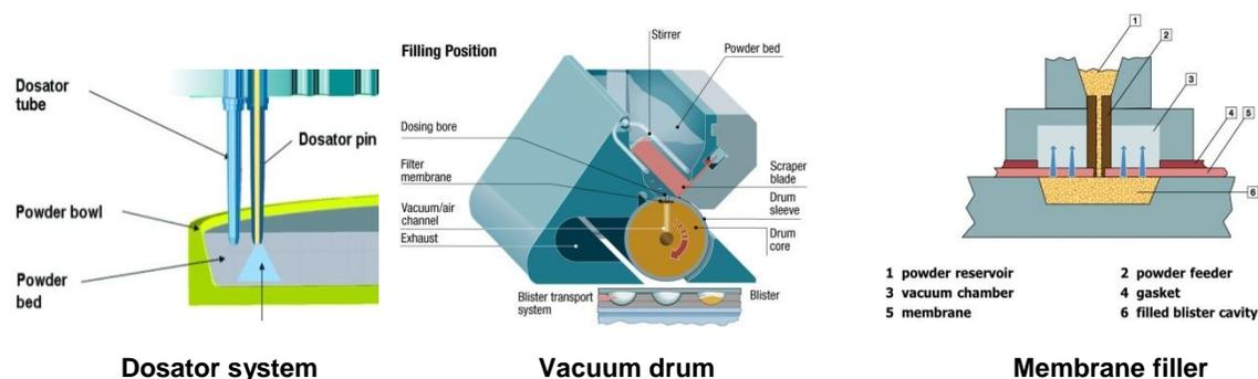
**Figure 1: Common microdosing systems to fill powder into inhaler disc cavities**
