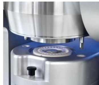
**Figure 5: Powder discharge into inhaler disc**
