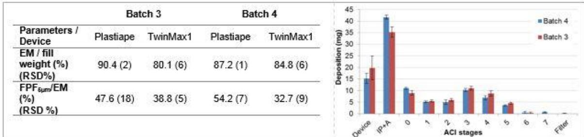
Figure 3 – Aerodynamic performance results of two replicate batches, when tested with TwinMax1 and with Plastiape.
