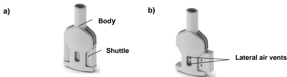
**Figure 1. The TwinMax™ concept: a) Perspective view with shuttle in storage position; b) Perspective view with shuttle in actuation position showing additional lateral air vents into the powder compartment.**
