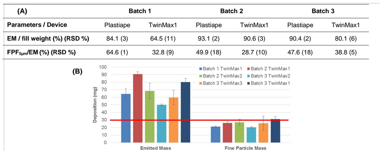
Figure 2 – (A) Aerodynamic performance of the 3 batches when tested with Plastiape and TwinMax1; (B) Comparison on the aerodynamic performance of several SD powders with different TwinMax prototypes (TwinMax1, TwinMax 2 and TwinMax 3).
