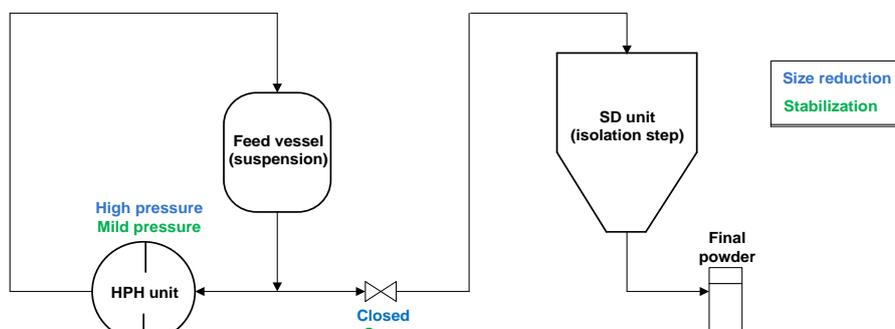
**Fig3.** Schematic representation of the Dynamic Suspension Drying (DSD) process.
