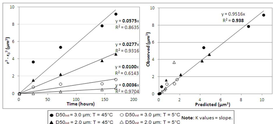
**Fig2.** Theoretical OR model versus experimental data (left plot) and observed versus predicted results (right plot)
