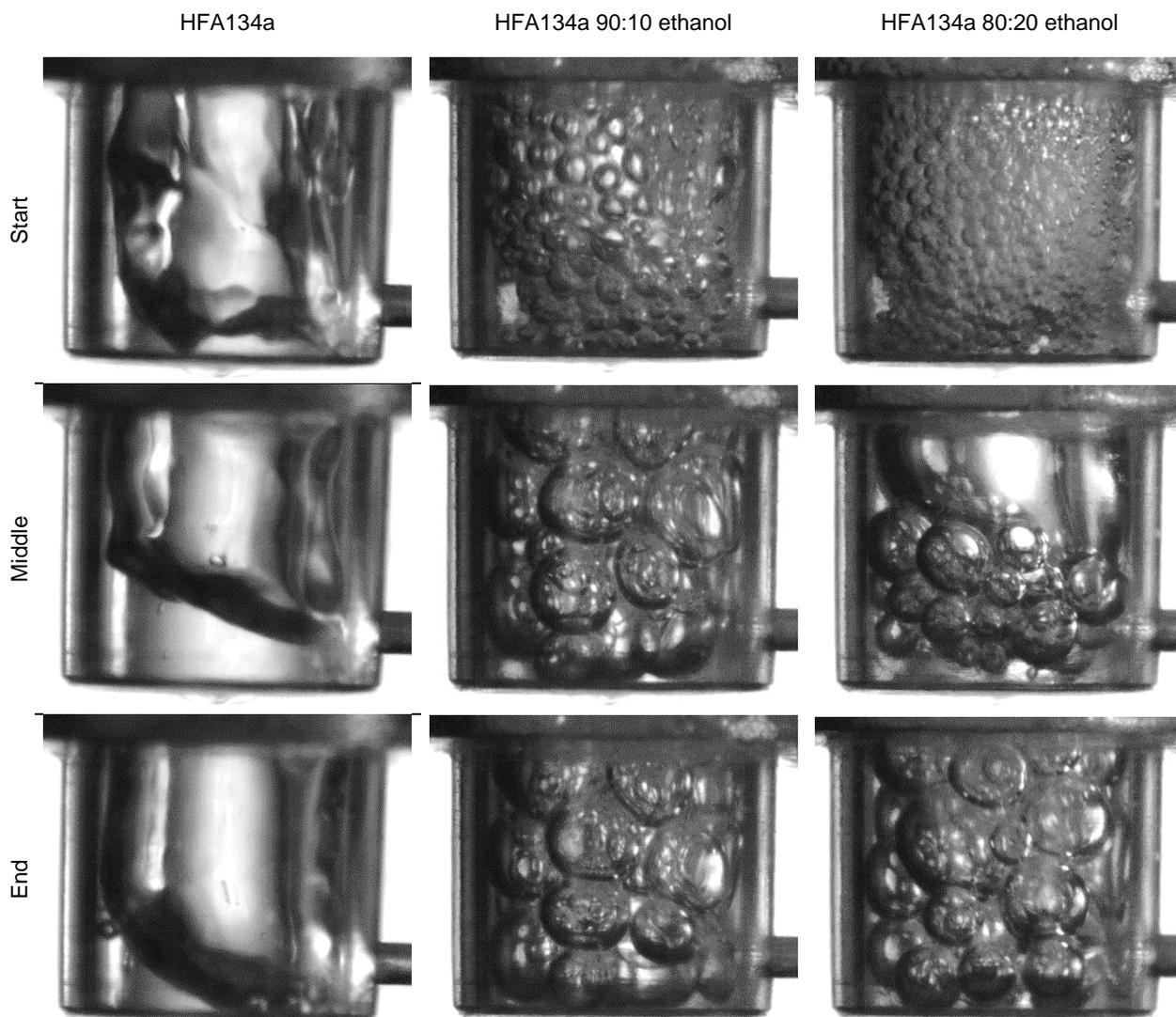
Figure 4 – Expansion chamber internal flow images. Formulations left to right; HFA134a, HFA134a 90:10 ethanol and HFA134a 80:20 ethanol. Event duration top to bottom; start middle and end of actuation event.
