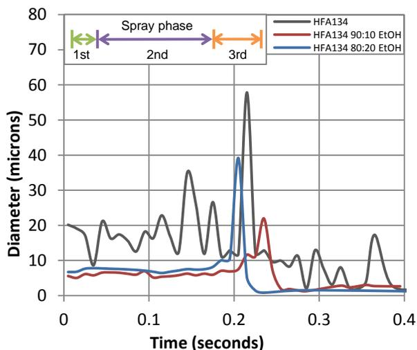
Figure 3 – Temporal variation of Sauter mean diameter of HFA134a/ethanol formulations
