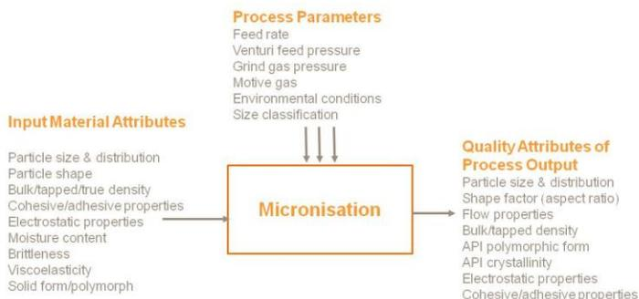
Figure 2. Input/Process/Output diagram for micronisation unit operation
