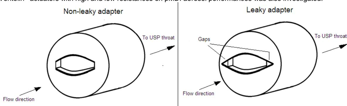
Figure 1 Schematic overview of the used adaptors
